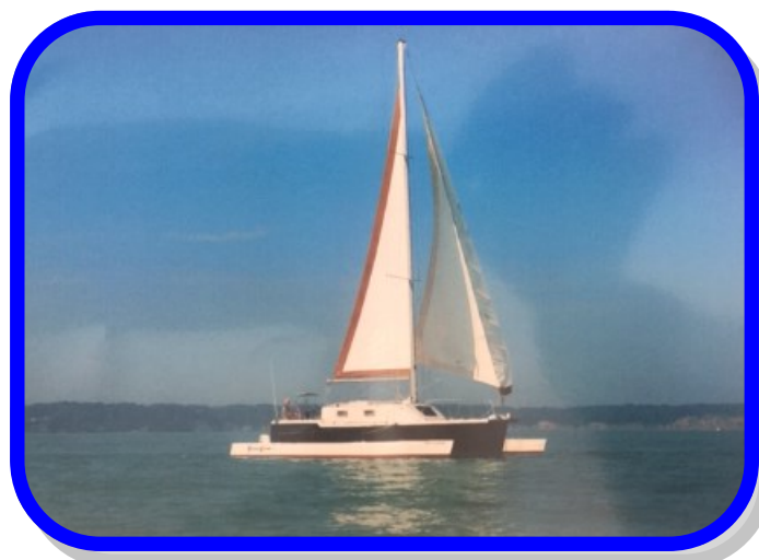
Another of Steve's 2 home made boats. This steel sail boat had folding out-riggers to increase stability, while allowing access to narrow channels and narrow docks.
